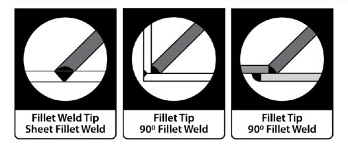
Fillet tips are used mainly for fillet welds [90°] and butt welds. The style of those tips allows one to weld from inside corners out and be able to seal the corners without changing to another tip style. Fillet tips can also be used for crack repairs, as long as the crack is somewhat straight. The longer preheat section allows faster welding speed than welding cracks with the conical tip.
