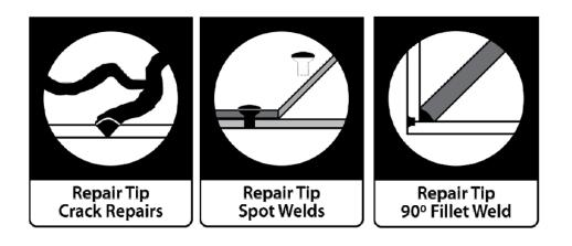
Repair tips are used for crack repairs, filling small holes, spot welding, for reaching tight areas, and for prototyping. Because of their conical shape, the repair tip and prototyping tip offer similar types of welds. Choose the size that best suits your application.
