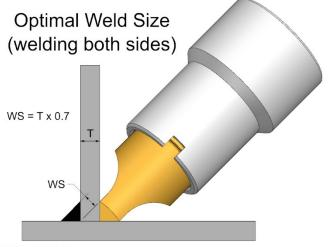
WS = Weld Size T = Plastic Thickness
